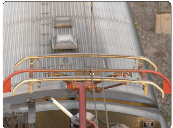
Photo of an undamaged pantograph on a train passing at 209 km/h.
